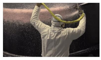
After applying the gelcoat surface and adding vinyl ester for corrosion and blister resistance, we focus on building strength into the pool shell with chopped fiberglass. We apply this material with a "chopper gun" that cuts long strands of glass fiber into pieces about an inch long. The gun also sprays resin and catalyst onto the mold while it chops fiberglass. Once chopped and sprayed, we roll out the fiberglass layer to strengthen it and remove any potential air bubbles.
